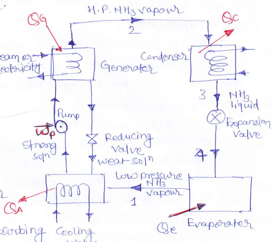
Strong solution rich in ammonia, is pumped (increasing the pressure of the solution upto condenser pressure) to the generator where heat ( $Q_G$ ) is supplied from an external source. Since the boiling point of ammonia is less than that of water, the ammonia vapour is given off from the aqua-ammonia solution at high pressure, and the weak solution returns to the absorber through a pressure reducing valve.
